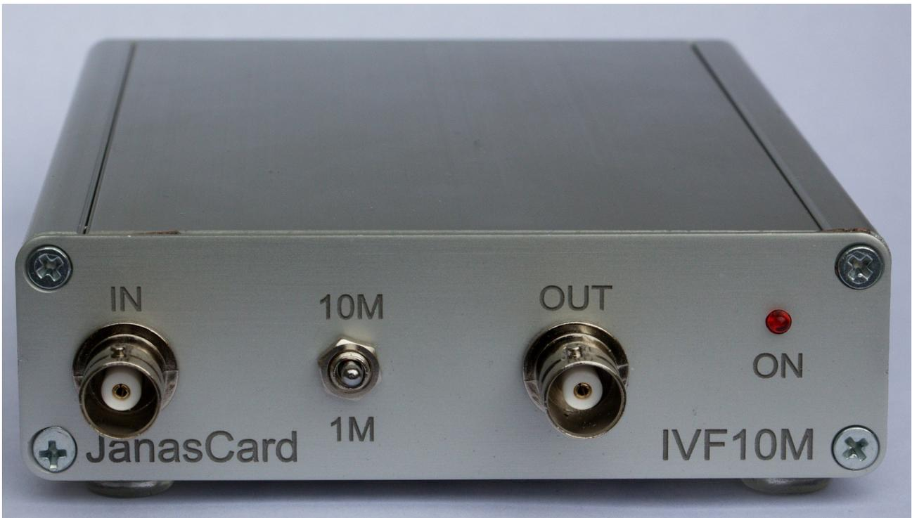
Figure 9. A practical example of a low noise hybrid TIA
