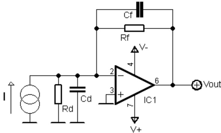
Figure 1. A basic transimpedance amplifier.
