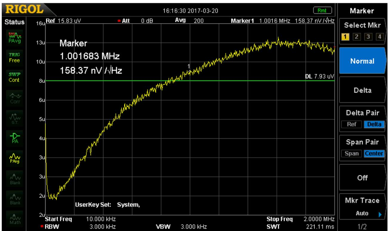
Figure 10. Output noise density of IVF10M at gain 1e6
