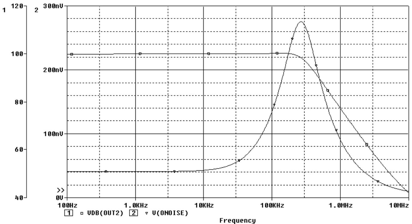
Figure 2. SPICE simulation of the TIA with OPA827.
